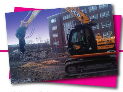
1,720 Joules at the tip of the steel for a 2:1 power to weight ratio. The 650 kg RH-4500 develops 4,500 Joules to deliver a thumping 7:1 power to weight ratio equivalent to seven Joules per kilogram.
